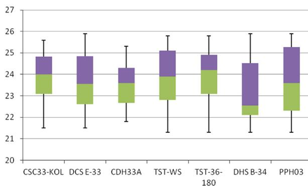
**Fig. 6 – Pressure resistance test. Graphic representing leak pressure values of all 50 anastomoses performed with each stapler. Different staplers are represented on the x-axis. Pressure values are expressed in kPa on the y-axis.**
